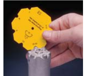
A useful tip: Use a Secoroc grinding template, and you'll see when it's time for a regrind.
